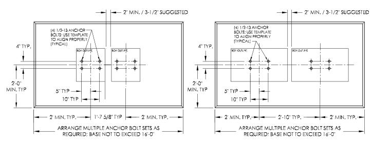
The Type II OPL has an identical box outline pattern as all six of the CBU types and therefore this configuration may also be used for one Type II OPL and one CBU if needed.
